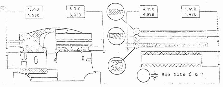
Piston Rings should be installed as shown above.
