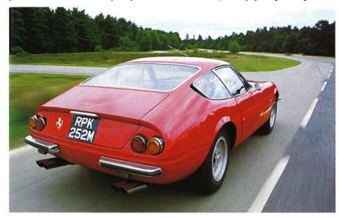
Muscular looks match 4.4-litre four-cam V12 with six Webers; one of few Ferraris not to use open gear gate; discreet doorhandle; flat steering wheel; flip-up lights from mid-'71, clear covers before
